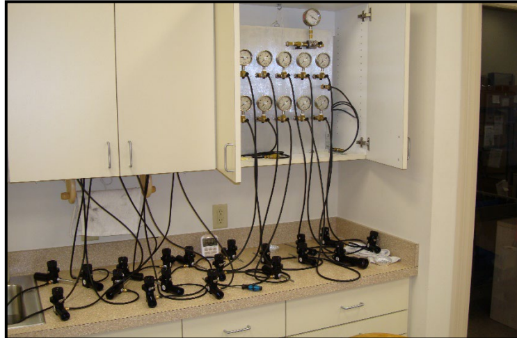
Illustration 4A: Graflex Nitrogen Test & Purge Bench
