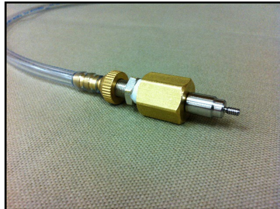
Illustration 4B & 4C: Camera Pressure Connector is screwed into “purge port” and pressure held for 2 hours at 2 psi.
