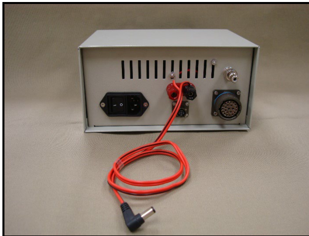
Illustration 2: BCA Camera/Cable Test Box
