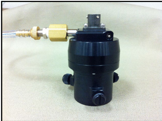
Illustration 4B & 4C: Camera Pressure Connector is screwed into “purge port” and pressure held for 2 hours at 2 psi.
