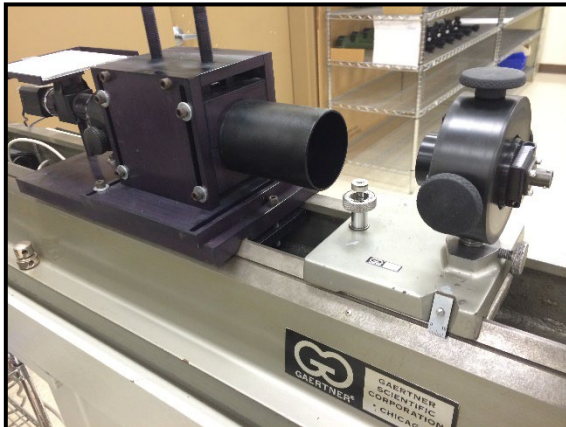
Illustration 1: BCA Camera Bench Fixture – Holds Camera firmly in one position for use on Graflex Optical Bench.
