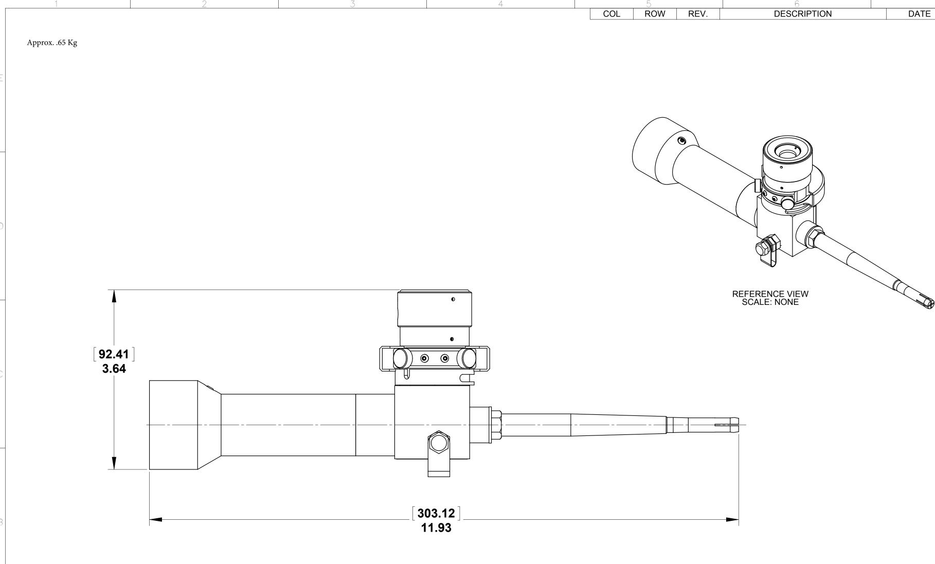
1. Standard integral 7.62mm stem is shown, non-standard lengths may be specified.
